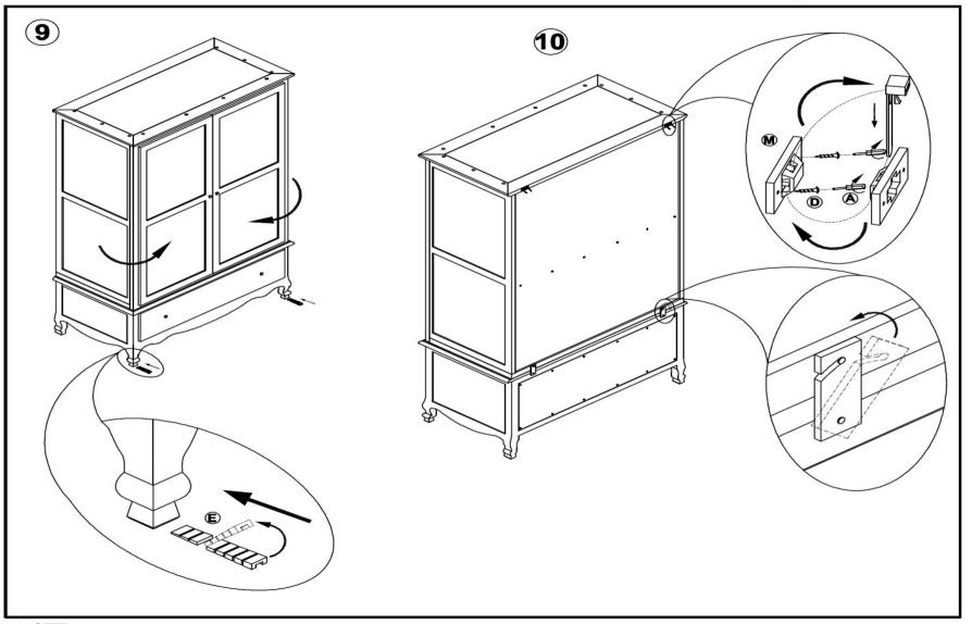
**NOTE:** IF THE UNIT IS NOT LEVEL, PLACE A LEVELER UNDERNEATH ONE FOOT UNTIL THE UNIT IS LEVEL. BREAK OFF ANY PROTRUDING SEGMENTS
